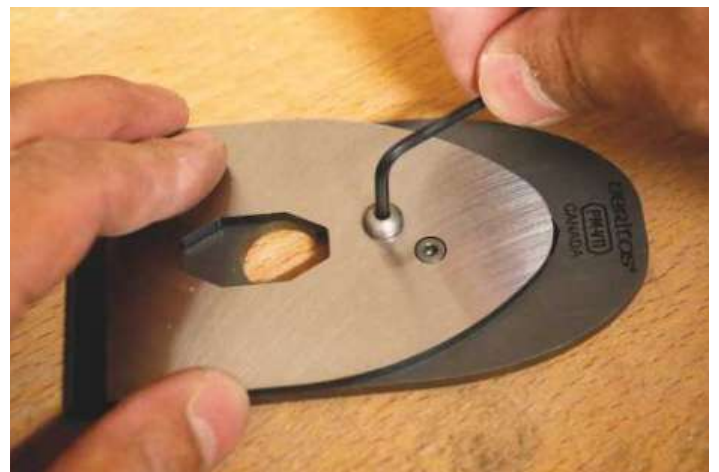
▲ Working on the iron requires the hex wrench
